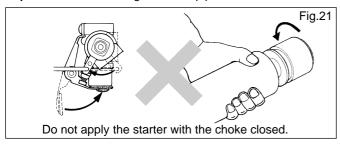
Warning! Never close the choke valve when applying the starter. Such an action will cause an excess quantity of fuel to be drawn into the cylinder and result in hydraulic lock that may damage the engine. (Fig.21)
