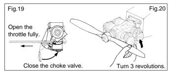
If very strong compression is felt when trying to turn the propeller counter-clockwise, too much fuel has been drawn into the engine. In this case, do not use force, but release the choke valve and turn the propeller clockwise slowly to eject excess fuel through exhaust pipes.
