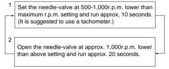
Repeat above procedure, i.e., richening and leaning the mixture until the engine has approx. 10 minutes of running time.
