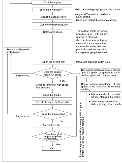
Attention: Do not leave the battery connected while adjusting the carburetor.
